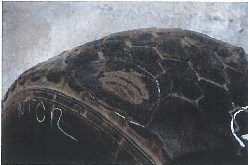
4. Casing rejected due to damage as deep as the wire breaker and damage on the belt edge.
