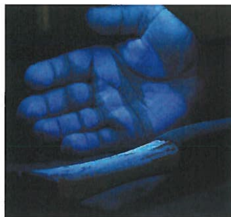
Figure 5: Hand (slightly creased with moisturizer) after one-time touching a rubber coated hammer shaft. The spots where PAHs were transmitted due to contact with the rubber fluoresce in UV light. Holes in the coating become visible.
