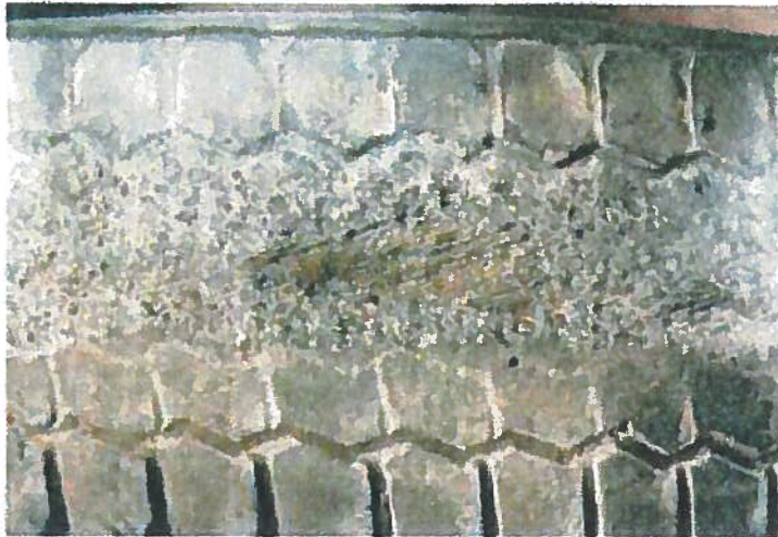
3. Casing rejected due to deep excess rust
